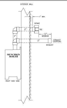
2" SIDEWALL VENT WITH TEE (INTAKE) & COUPLING (EXHAUST) FOR T50M/T80M WALL MOUNTED UNITS
